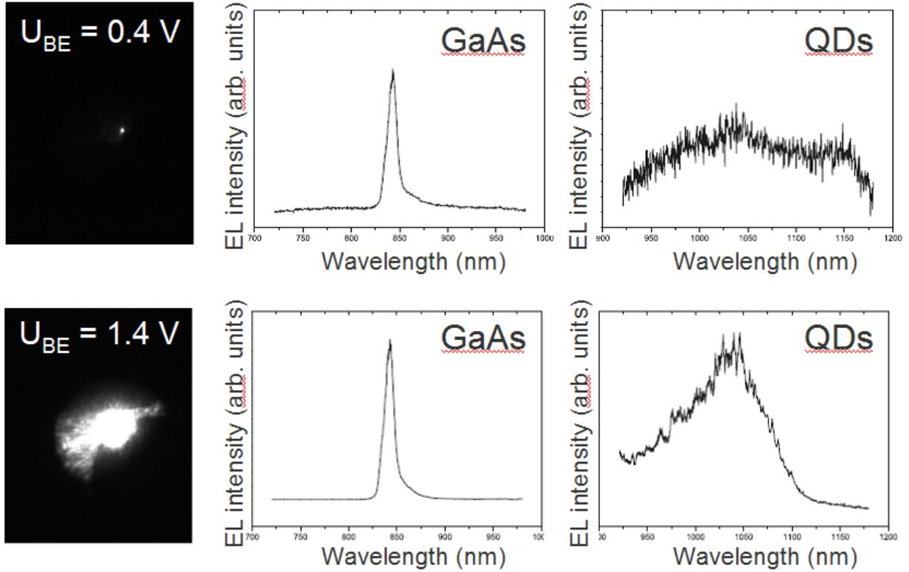
Fig.9: Low-temperature ( $T = 5$  K) electroluminescence of a spin-injection transistor: CCD images (left) and corresponding spectra in the wavelength range of GaAs (middle) / QD emission (right). The top and bottom row show results for two different base-emitter voltages  $U_{BE}$ . The collector-emitter voltage was fixed at  $U_{CE} = 2$  V.
