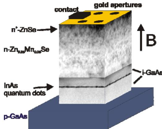
Fig.1: Schematic set-up of a spin-LED. n-type ZnMn(S)Se:Cl is used as a spin aligner for electrons in an applied magnetic field. The optically active InGaAs QDs are embedded in the intrinsic part of the p-i-n structure. The LED is etched from the plane sample as a mesa and contacted by In and a gold wire. The upper surface is covered with a gold layer containing nano-apertures for single-dot spectroscopy [A2.3:20,12].
