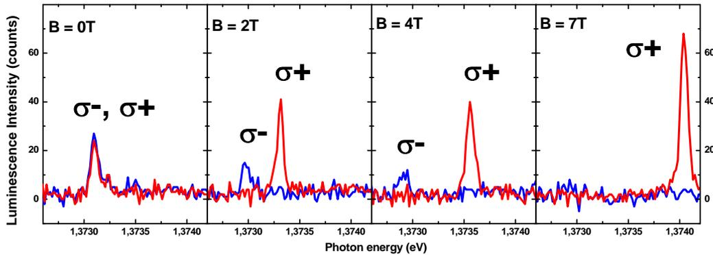
Fig.3: Intensity of the (circularly polarized) electroluminescence from the Zeeman-split ground-state doublet of a single QD. After [A2.3:20].
