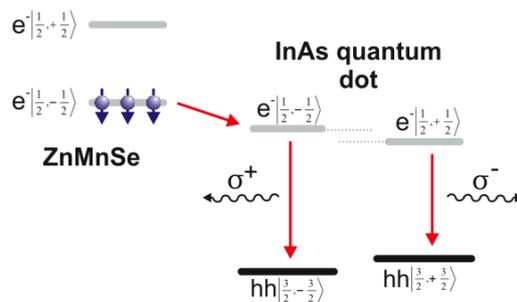
Fig.2: Schematic diagram of the electron levels in the spin aligner and the QDs. Injection of electrons into the dots leads to circularly polarized luminescence. The polarization degree is a function of the spin orientation in the dots.
