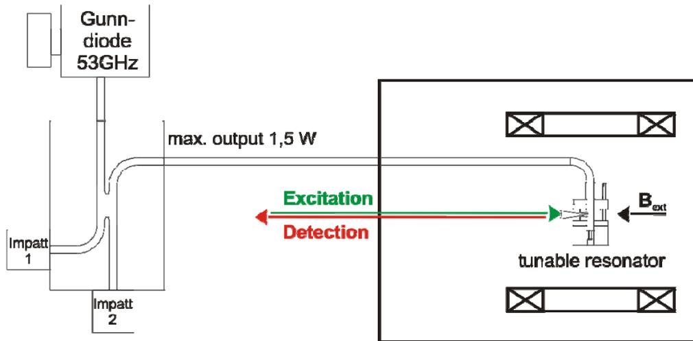
Fig.10: Microwave source and cryostat with resonator. The radiation from the amplified Gunn source at 53 GHz is guided into the cryostat where the external magnetic field is applied. Optical access to the sample is provided by a detection hole in the microwave resonator.
