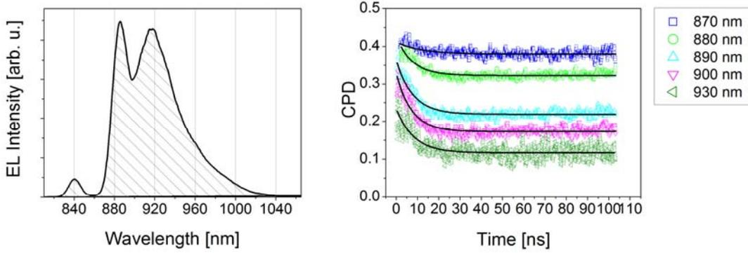
Fig.5: Left: EL spectrum of a spin-LED at  $T = 5$  K. The GaAs-related emission is centered at 840 nm. The wetting layer emission exhibits a peak at 885 nm, the QD emission can be observed at higher wavelengths. Right: Time-dependent CPD ( $T = 5$  K,  $B = 6$  T) for several wavelengths at time  $t$  after the beginning of the EL signal. Lower curves represent higher wavelengths. Solid lines are exponential fits [A2.3:32].
