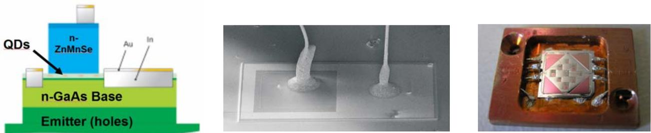
Fig.8: Left: Schematic design of our spin-injection transistor. Middle: Scanning electron microscopy image of contacted structure. Right: Photograph of the mounted device.
