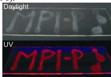
Fig.6: Luminescence of the 2b in a matrix of polylaurylmethacrylate (PLMA).
