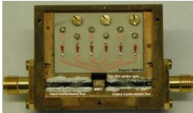
Fig. 7: Micrograph of the housed MMIC. The size of the gold-coated brass housing is 33 \times 40.6 \text{ mm}^2 . The connection with the external electrical network is realized by two SMA connectors.
