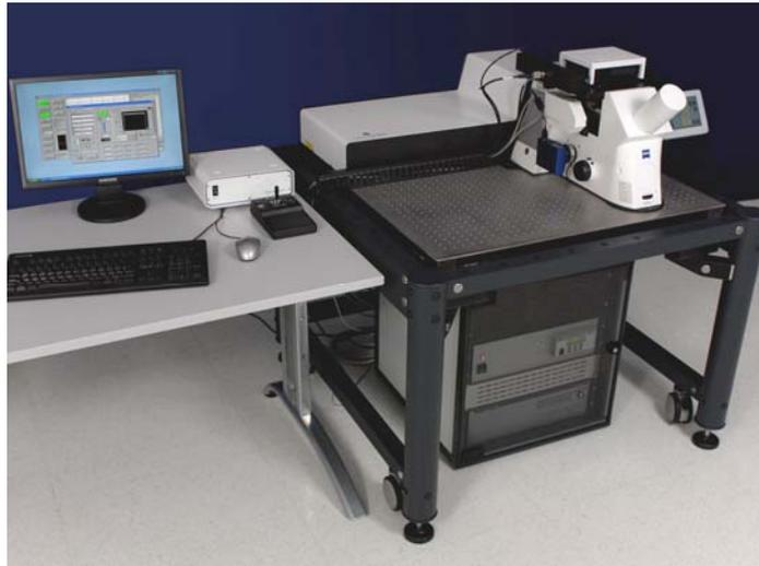
Fig.1: The three-dimensional optical lithography system commercialized by the start-up company Nanoscribe GmbH, which emerged out of CFN subproject A1.4. Nanoscribe GmbH was officially founded in December 2007. In 2008, Carl Zeiss AG acquired nearly 40% of the shares of Nanoscribe GmbH.
