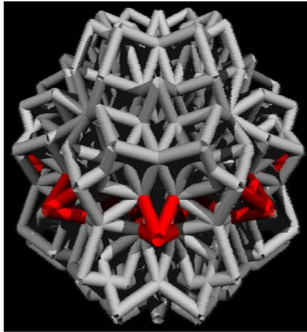
Fig.7: Scheme of part of a three-dimensional rhombicuboctahedral quasicrystal. The local eight-fold rotational symmetry is highlighted in red. Taken from Ref.[A1.4:25], where our fabricated structures have also been presented.
