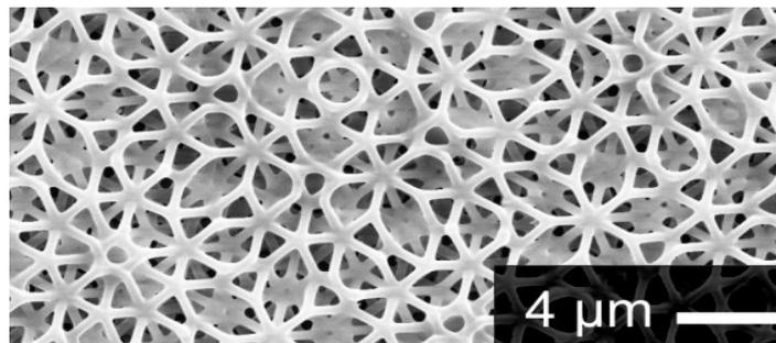
Fig.6: Top-view electron micrograph of a 3D icosahedral photonic quasicrystal. Note the local five-fold symmetry axis. Taken from Ref.[A1.4:7].
