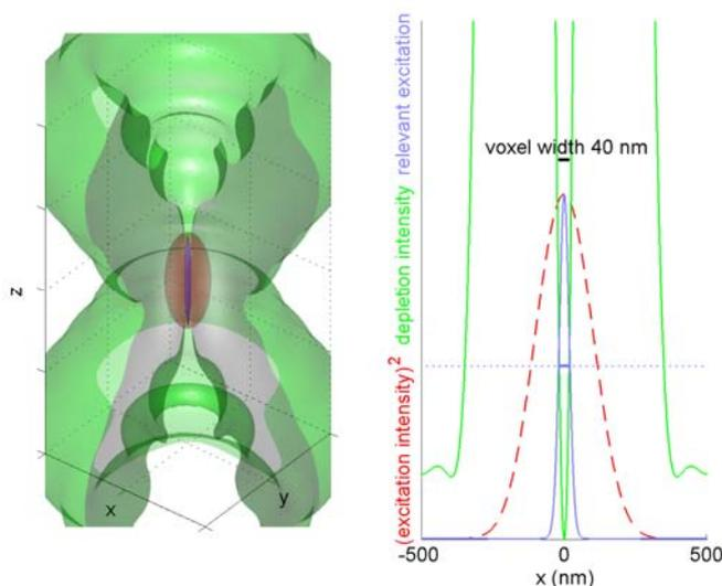
Fig.9: Illustration of the foci of light used in lateral STED-DLW in 3D (left panel). The red profile excites, the green profile depletes, leading to the effective dose profile shown in blue. The right panel shows a cut through the focal plane. Parameters are 810 nm wavelength of light (red) for the excitation, 532 nm (green) for the depletion, and a microscope lens numerical aperture of  $NA=1.4$ . Taken from Ref.[A1.4:27].
