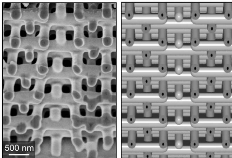
Fig.3: Electron micrograph of a vertical waveguide within a three-dimensional silicon photonic-band-gap structure after focused-ion-beam milling to reveal the interior (left) and corresponding scheme (right).
