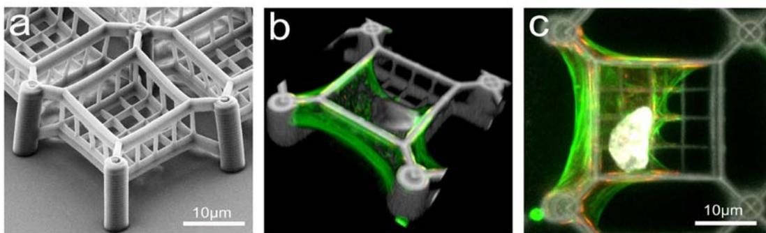
Fig.7: Example of a 3D *ORMOCER* template structure fabricated via DLW in A1.4 for biological cell growth studies in CFN subproject E2.3. Taken from Ref.[A1.4:22].
