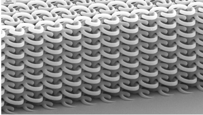
Fig.5: Electron micrograph of a fabricated bi-chiral photonic crystal. Taken from Ref.[A1.4:19].
