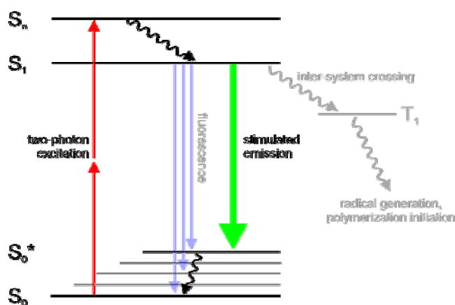
Fig.8: Jablonski diagram of a photoinitiator molecule. Taken from Ref.[A1.4:27].
