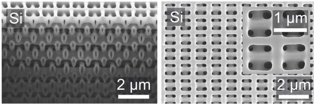
Fig.2: Electron micrographs of a 3D silicon woodpile photonic-band-gap material made via DLW and the silicon double-inversion procedure introduced within subproject A1.4. The left panel shows a focused-ion beam cut to reveal the 3D interior, the right panel a top view. Taken from Ref.[A1.4:1].
